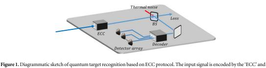
Figure 1. Diagrammatic sketch of quantum target recognition based on ECC protocol. The input signal is encoded by the 'ECC' and prepared as the emitted state to illuminate the object modeled as a beam splitter (BS). The reflected signal is injected into the decoder and then be detected by the detection array.
