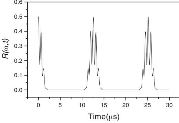
**Figure 1.** The module  $R(\omega, t)$  of the off-diagonal element of the density operator is plotted as a function of time with a fixed trap frequency. The parameters chosen are  $\alpha_g = \alpha_e = 3$ ,  $\omega = 2\pi \times 11.3$  MHz,  $\delta = 4$  GHz,  $\Omega_L = 10$  kHz.
