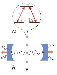
FIG. 1. (Color online) The cavity QED model of our QHE. Three-level atoms, with quantum coherence in the two degenerate ground states  $|g_1\rangle$  and  $|g_2\rangle$ , flow through the cavity and interact with the resonant photon field in the cavity.
