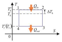
FIG. 2. (Color online) Temperature-entropy diagram for the photon-Carnot cycle. Here we consider neither the cavity loss nor the atomic dephasing. i.e.,  $\xi = 1, Q \rightarrow \infty$ . In addition, we consider the special case of the phase angle  $\operatorname{Arg}(c_1c_2^*) = \pi$ . As a result the effective temperature  $T'_h$  is higher than  $T_h$  by the amount  $\Delta T_h = n_h T_h |c_1^h c_2^{h*}| / P_e^h$ .
