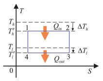
FIG. 3. (Color online) Temperature-entropy diagram for the photon-Carnot cycle. The atomic coherence is demolished due to the atomic dephasing, i.e.,  $\xi=0$ . The cavity loss makes the effective cavity temperature decrease. Here,  $\Delta T_h = n_h T_h \nu_h / (2\mu P_e^l Q)$ , and  $\Delta T_l = n_l T_l \nu_l / (2\mu P_e^l Q)$ .
