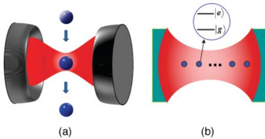
FIG. 1. (Color online) (a) Schematic diagram of our single particle thermalization model that a series of prepared TLSs randomly pass through a single-mode cavity one by one, in equilibrium it is equivalent to the conventional reservoir model, (b) where many identical atoms with spatially random distribution thermalize the single-mode cavity field.
