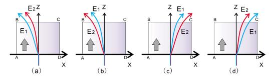
FIG. 2. (Color online) Schematic illustration of the asymmetric deflection of probe light by the nonuniform magnetic field in conditions (a)–(d).
