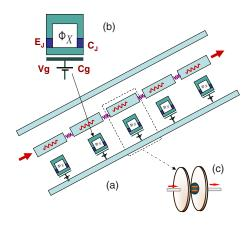
FIG. 1. (Color online) Configuration of the setup for controlling light propagation in a coupled-line-resonator waveguide (a) by coupling to charge qubits (b). The coupled (line resonators)–(charge qubits) system can behave similarly to the cavity QED for a single atom interacting with a single-mode cavity (c).
