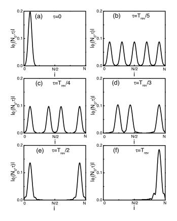
FIG. 3. The illustrations of the fractional revival via the time evolution of a GWP with  $\Delta = 24$ ,  $N_0 = 50$  in the system with N = 500. (a)  $\tau = 0$ , (b)  $\tau = T_{rev}/5$ , (c)  $\tau = T_{rev}/4$ , (d)  $\tau = T_{rev}/3$ , (e)  $\tau = T_{rev}/2$ , (f)  $\tau = T_{rev}$ . It shows that at  $\tau = T_{rev}p/q$ , the GWP splits into several sub-GWPs at corresponding positions with the same shape as the initial one.
