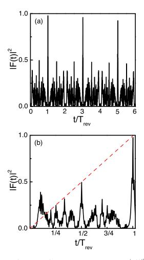
FIG. 2. (Color online) Plots of the square of fidelity,  $|F(t)|^2$ , for the initial GWP with  $\Delta = 24$ ,  $N_0 = 50$  in the system with N = 500. (b) is a part of (a) over one revival time. The dashed line indicates that the square of the fidelities at  $\tau/T_{rev} = 1/2$ , 1/3, 1/4,... are approximately in a line.
