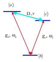
FIG. 1. (Color online) Three-level cyclic atoms are resonantly coupled to two quantized fields and a classical field via electricdipole interaction.
