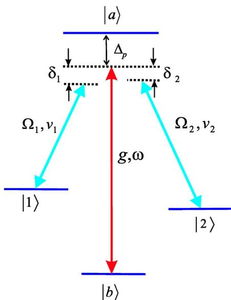
FIG. 1. Four-level atom interacting with a quantum probe field (with coupling constant  $g$ , frequency  $\omega$ , and the detuning  $\Delta_p$ ) and two classic control fields (with frequency  $\nu_k$ , coupling Rabi frequency  $\Omega_k$ , and the detuning  $\Delta_k = \omega_{ak} - \nu_k$ ,  $k=1,2$ ). When  $\delta_k$  ( $=\Delta_k - \Delta_p$ ) are very tiny, the system satisfies the near 3-photon resonance EIT condition.
