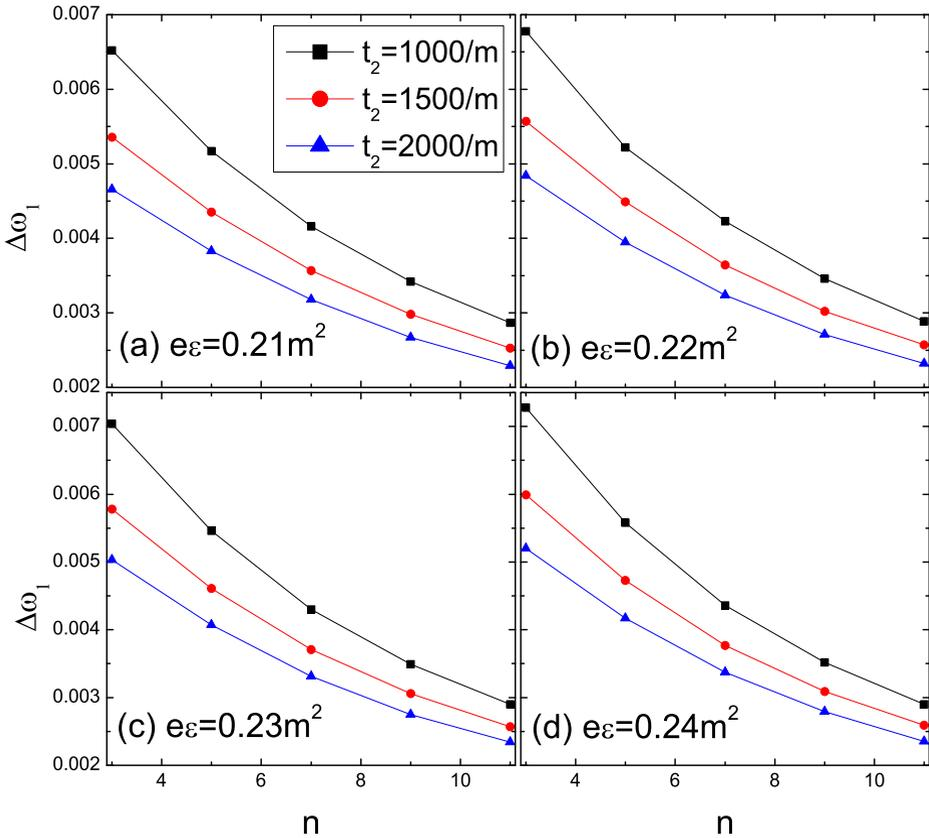
**Fig. 5** (Color online) With different strength of external field, we extract the sub-band width  $\Delta\omega_1$  as a function of the photon number  $n$ , (a)  $e\varepsilon = 0.21m^2$ , (b)  $e\varepsilon = 0.22m^2$ , (c)  $e\varepsilon = 0.23m^2$ , and (d)  $e\varepsilon = 0.24m^2$ . We can see the sub-band width decreases as photon number is increasing
