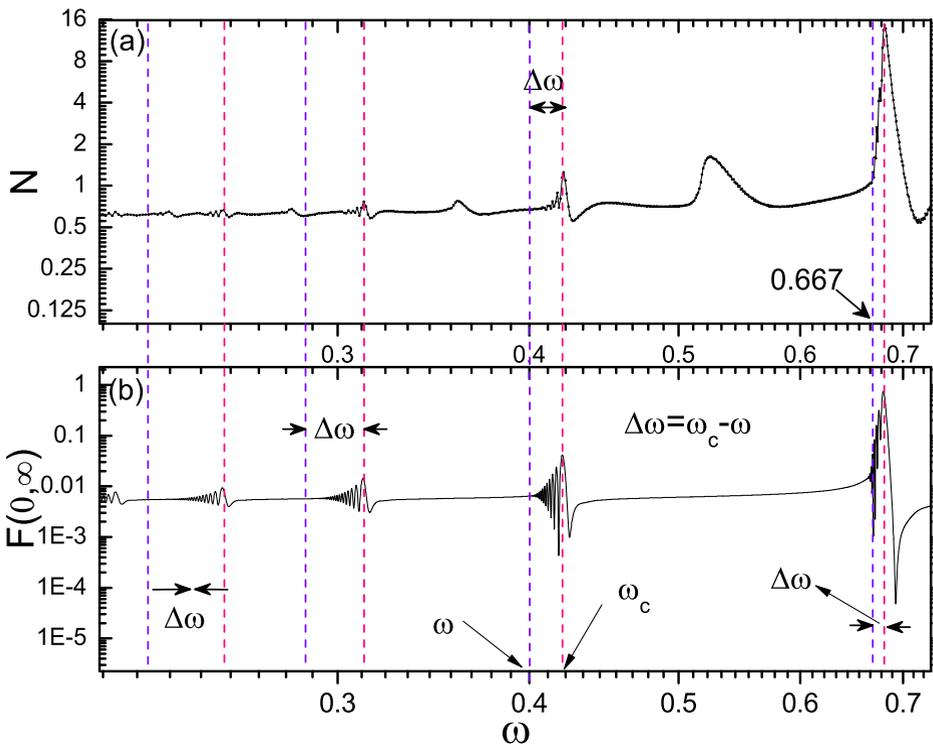
**Fig. 1** (Color online) **a** Log-plot of the particle yield for Half-Ladder shaped pulse,  $t_1 = 100/m$ ,  $t_2 = 2000/m$ , and  $e\varepsilon/m^2 = 0.20$ . **b** One-particle distribution in momentum space. The vertical dashed red lines denote positions of the true frequency  $\omega_c$ , the vertical dashed purple lines are the estimated threshold frequency  $\omega$ .  $\Delta\omega = \omega_c - \omega$  is the frequency shift
