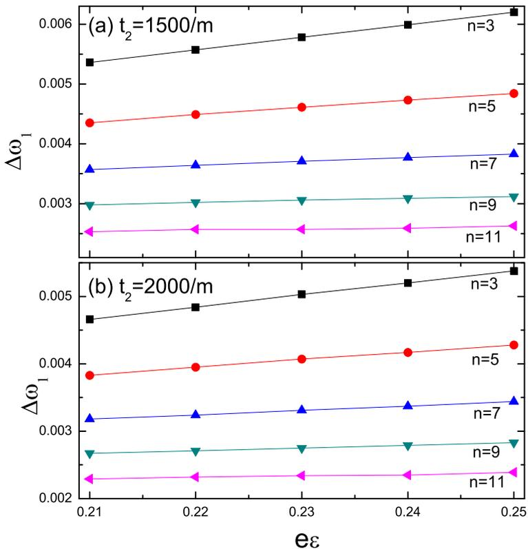
**Fig. 6** (Color online) With different pulse duration  $t_2$ , we extract the sub-band width  $\Delta\omega_1$  as a function of the strength of external field  $e\varepsilon$ , **(a)**  $t_2 = 1500/m$  and **(b)**  $t_2 = 2000/m$ . It is shown that the sub-band width increases as strength of external field is increasing
