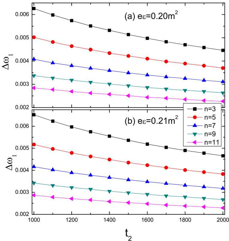
**Fig. 4** (Color online) With different  $e\varepsilon$ , we extract the sub-band width  $\Delta\omega_1$  as a function of the pulse duration  $t_2$  (scaled by  $m$ ) for different photon number, (a) for  $e\varepsilon = 0.20m^2$ , (b) for  $e\varepsilon = 0.21m^2$ . It is found that the sub-band width is decreases as  $t_2$  increasing and it is relatively larger for the lower photon number
